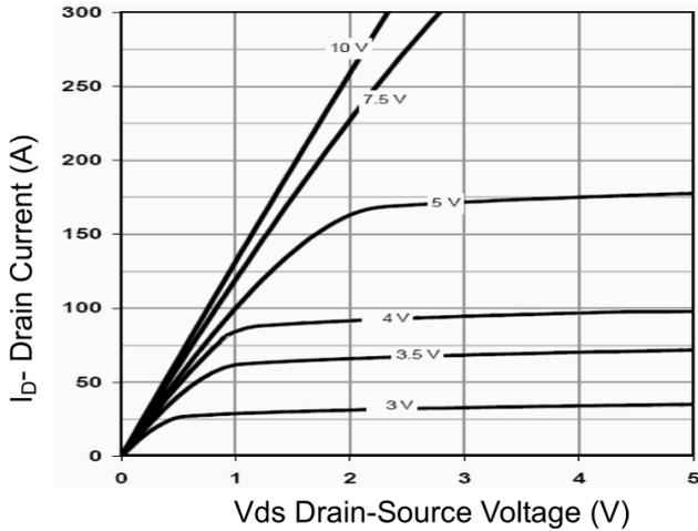
**Figure 1 Output Characteristics**
