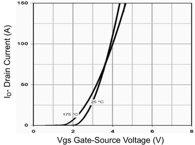
**Figure 2 Transfer Characteristics**
