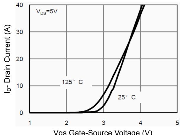
Figure 2 Transfer Characteristics
