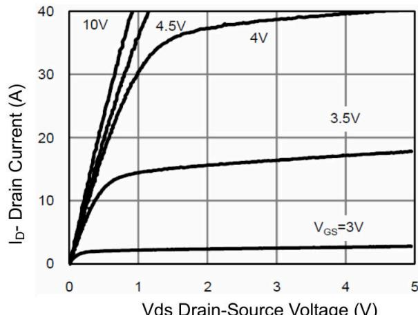
Figure 1 Output Characteristics
