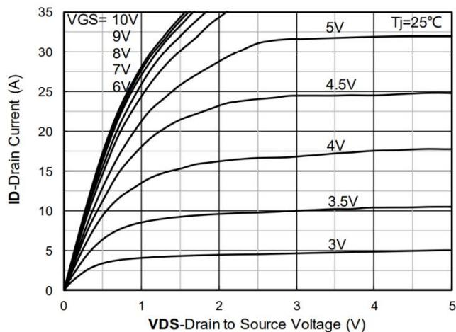
Figure 1. Output Characteristics
