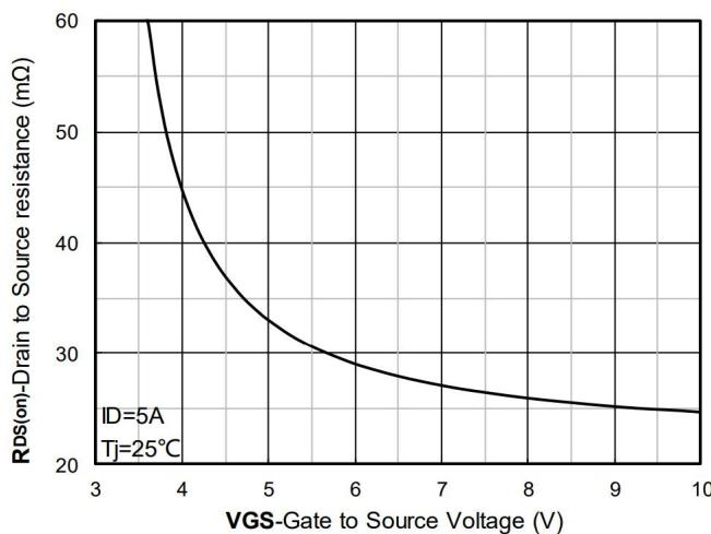
Figure 5. On-Resistance vs Gate to Source Voltage
