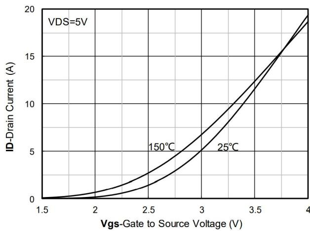
Figure 2. Transfer Characteristics
