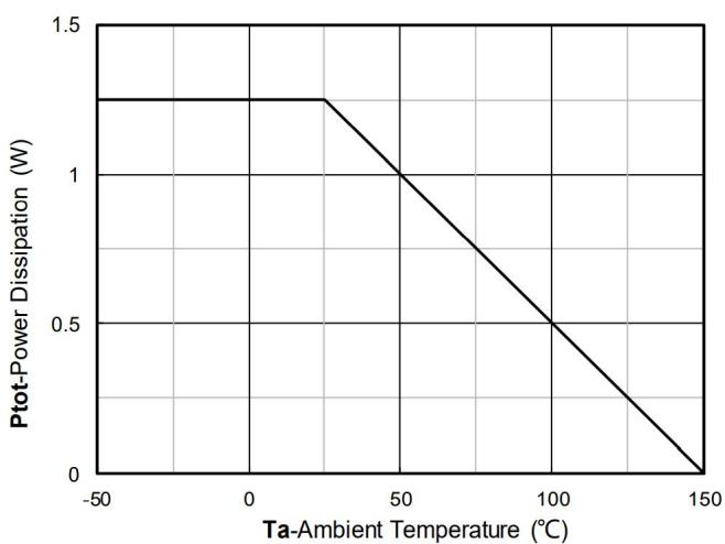
Figure 12. Power dissipation
