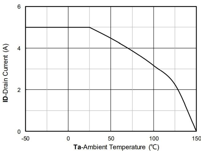
Figure 11. Current dissipation
