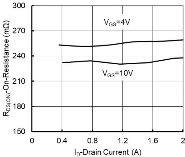
Figure 3: On-Resistance vs. Drain Current and Gate Voltage
