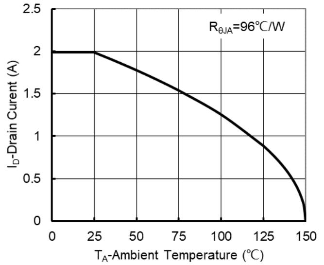
Figure 8. Maximum Continuous Drain Current vs Ambient Temperature
