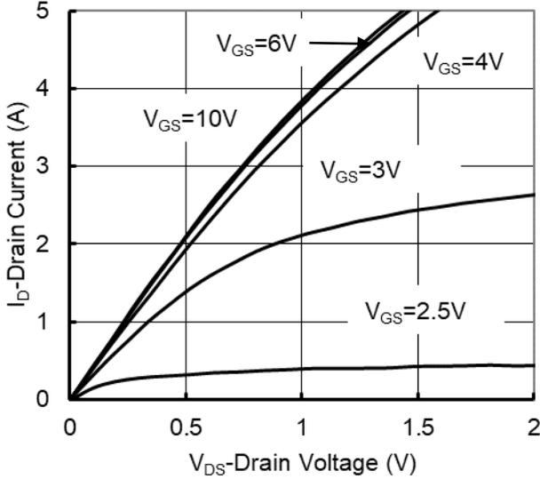
Figure1. Output Characteristics
