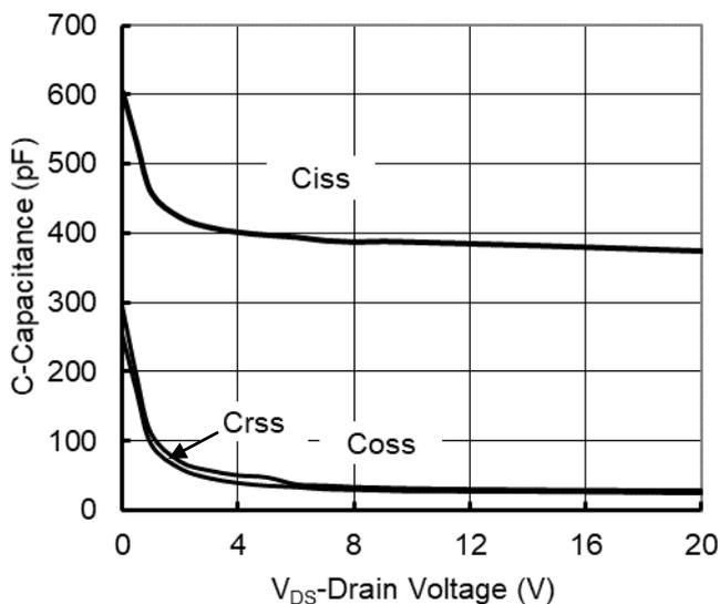
Figure5. Capacitance Characteristics
