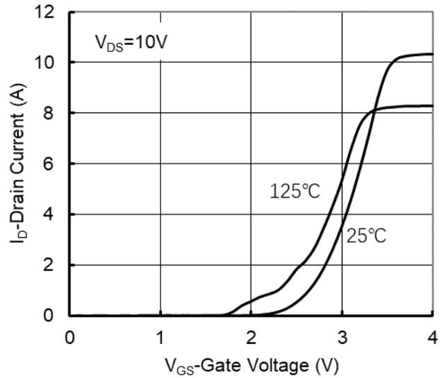
Figure2. Transfer Characteristics
