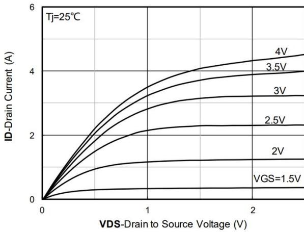
Figure 1. Output Characteristics
