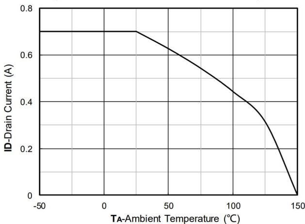
Figure 11. Current dissipation
