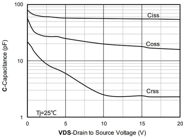
Figure 3. Capacitance Characteristics
