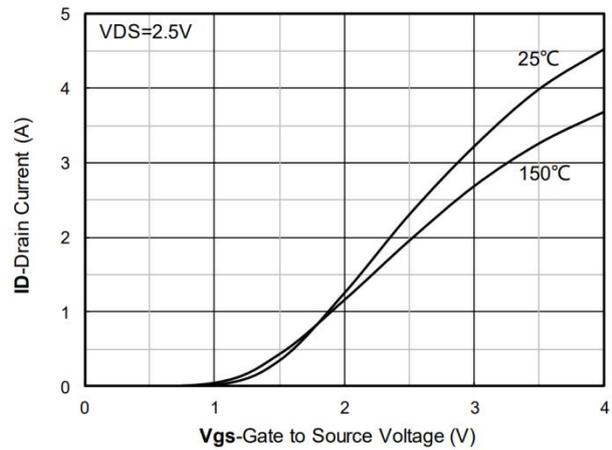
Figure 2. Transfer Characteristics
