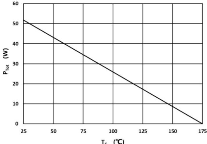
Figure 6. Power dissipation as function of case temperature
