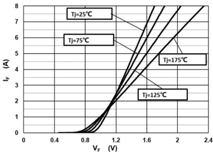
Figure 1. Typical forward characteristics
