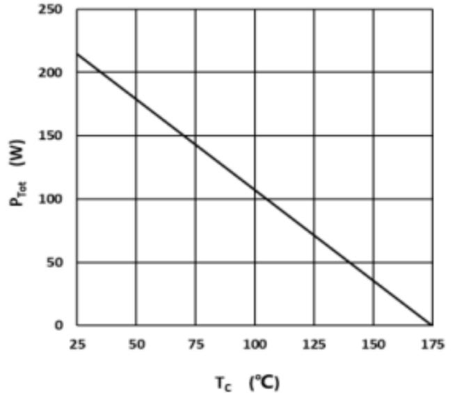
Figure 6. Power dissipation as function of case temperature
