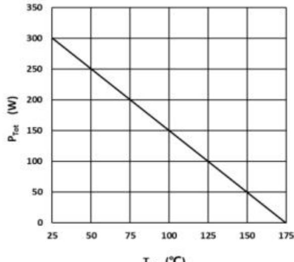
Figure 6. Power dissipation as function of case temperature
