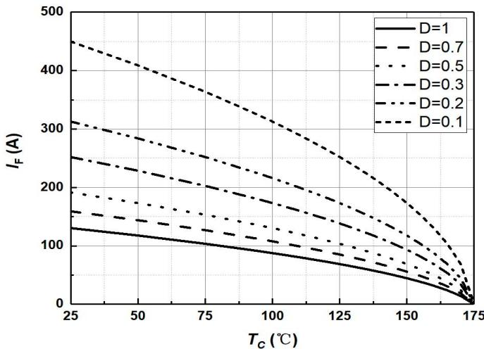
Figure 3. Diode forward current as function of temperature
