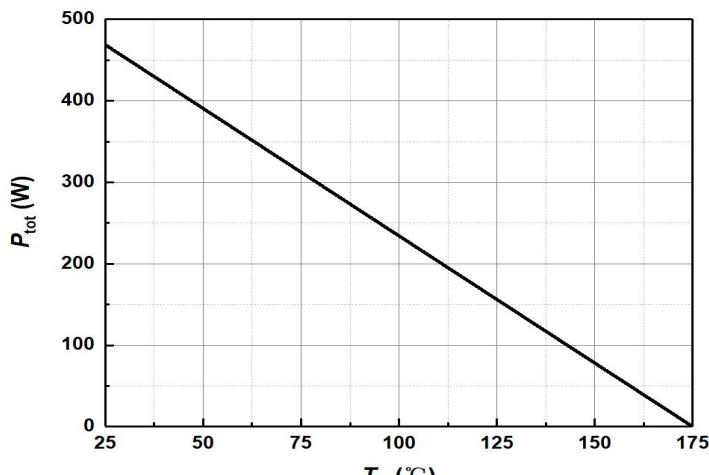
Figure 6. Power dissipation as function of case temperature
