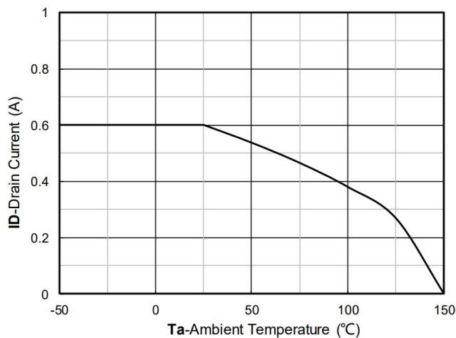
Figure 11. Current dissipation
