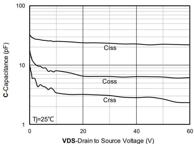
Figure 3. Capacitance Characteristics
