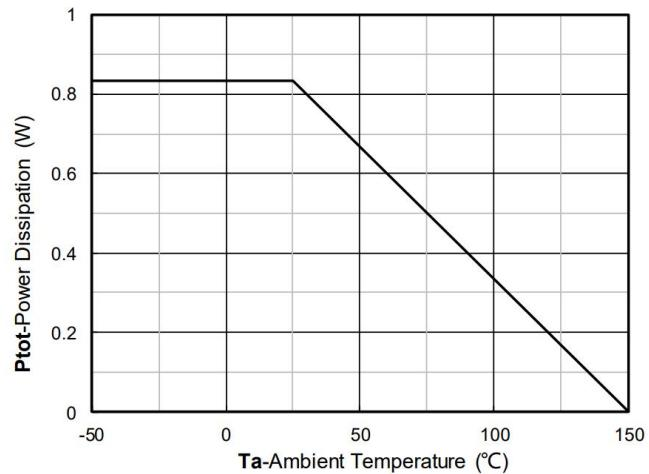
Figure 12. Power dissipation
